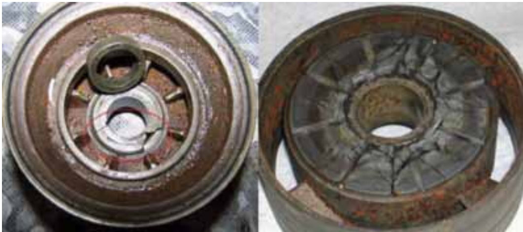
Figure 4—Carbide parts crack through thermal event
