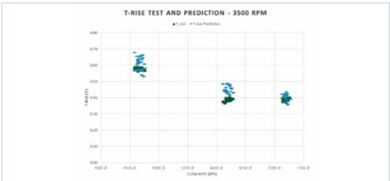
Figure 12—Good agreement on T-rise measurement and prediction using Equation 3
