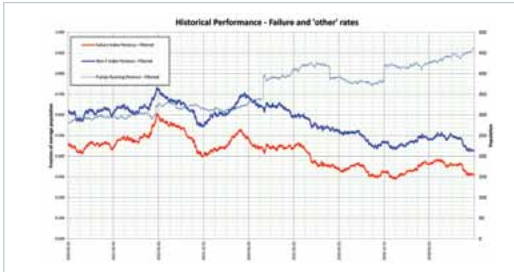
Figure 5—Failure and total 'Stop' indices vs. time for Perenco. On the right vertical axis, the number of operable ESP's.
