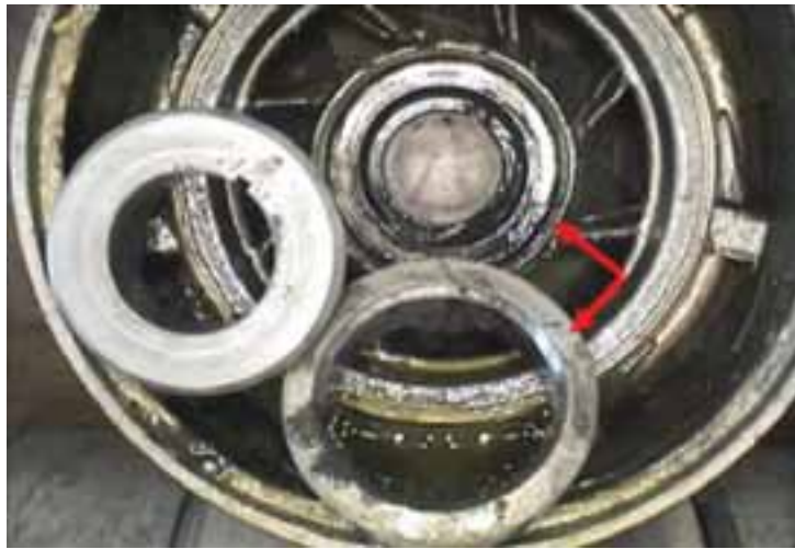
Figure 3—Carbide bushing insert loose and unseated from diffusers
